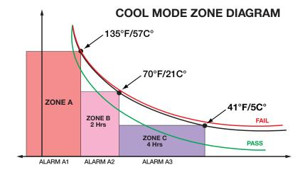
temperature to 70° F(21°C) within 2 hours and then from 70°F to 41°F(21°C to 5°C) within four hours to ensure safety. This model's unique, programmable three-zone cool down feature conforms to FDA Food Code 3-501.14 (A,B).
